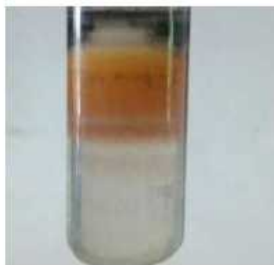
Figure 1 Mn doped crystals of Bismuth tri sulphide inside the test tubes
