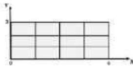
Figure 2: Finite difference arrangement for heat conduction problem.
