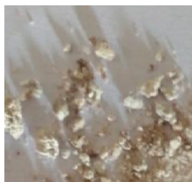
Figure 2 Manganese doped crystals of Bismuth tri sulphide outside the test tubes
