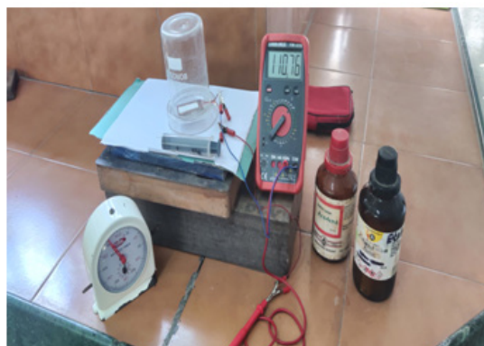
Fig. 4: Photograph of indigenously developed static gas sensing unit operating at room temperature.
