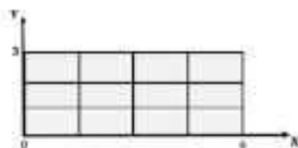
Figure 2: Finite difference arrangement for heat conduction problem.
